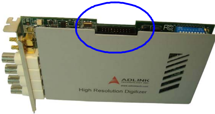
Figure 3-19: SSI Connector Location on the PCI-9816/26/46
