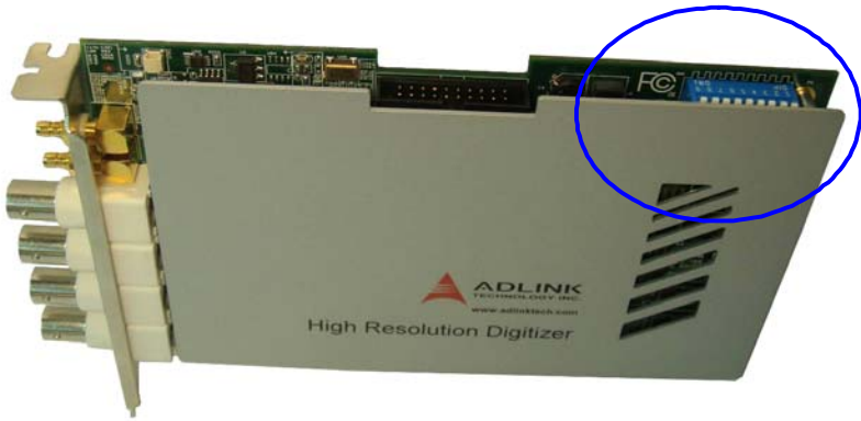
Figure 3-25: The Location of Board ID Switch
