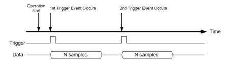
Figure 3-9: Re-Trigger Mode Acquisition
