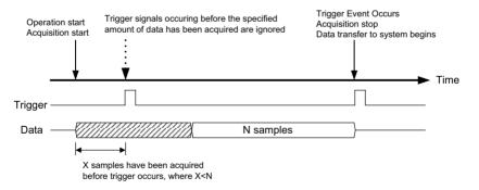
Figure 3-7: Pre-Trigger Mode Acquisition
