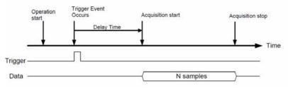
Figure 3-6: Delayed Trigger Mode Acquisition
