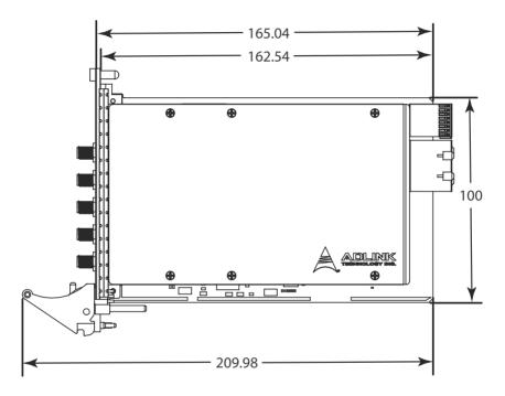
Figure 1-3: PXIe-9852 Schematic
