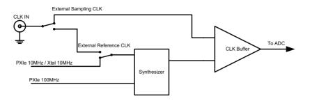
Figure 3-10: PXIe-9852 Clock Architecture
