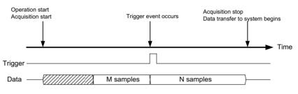
Figure 3-8: Middle Trigger Mode Acquisition
