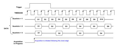
Figure 3-13: Varying Sampling Rates by Adjusting Scan Interval Counter
