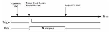
Figure 3-5: Post-Trigger Acquisition
