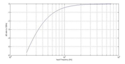
Figure 1-2: Magnitude Response of AC Couple of Input Channel
