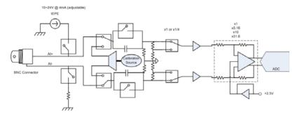
Figure 3-1: Analog Input Architecture of the PXI-9527
