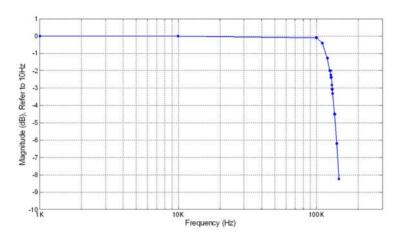
Figure 1-1: Analog Input Channel Bandwidth, ±10 V Input Range
