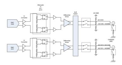
Figure 3-3: Analog Output Architecture of the PXI-9527
