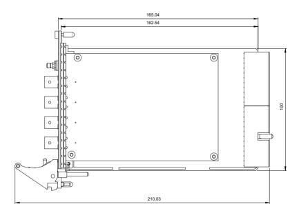
Figure 2-1: PXI-9527 Side View
