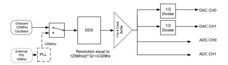
Figure 3-9: PXI-9527 Timebase Architecture
