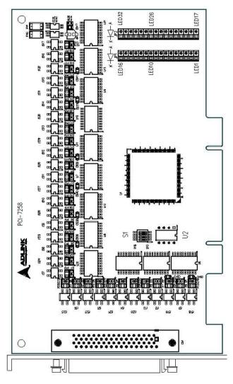
Figure 1: PCI-7258 PCB Layout
