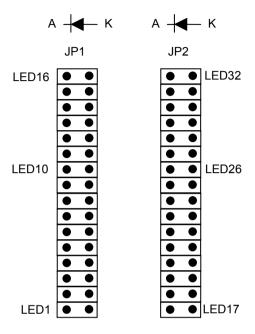
Figure 2: PCI-7258 External LED connector
