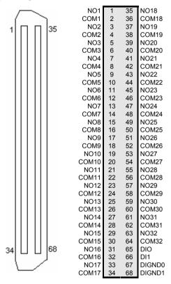
Figure 4: Pin Assignment of PCI-7258 CN1
