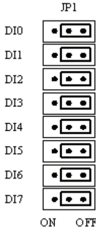
Figure 2-2: Default Input Signal Jumper Setting
