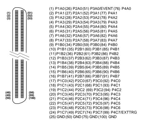
Figure 2.3 Connectors Pin Assignment of PCI-7396
