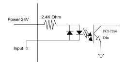
Figure A1.1: opto-isolated input circuit
