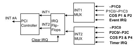
Figure 4.4 Dual Interrupt System of PCI-7396
