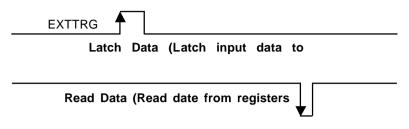
Figure 4.2 Read Data use External Trigger
