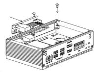
5. Connect PCM IO module with mini-PCIe card and power connector on MB via cable.
