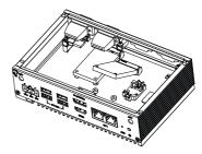
3. Remove the screws to remove the blank expansion plate.
