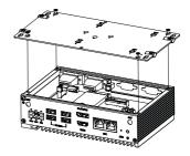
2. Insert the mini-PCIe card and secure the screws.
