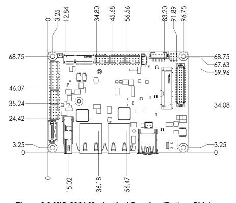
Figure 2.3 MIO-2361 Mechanical Drawing (Bottom Side)
