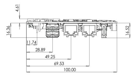
Figure 2.4 MIO-2361 Mechanical Drawing (Side View)
