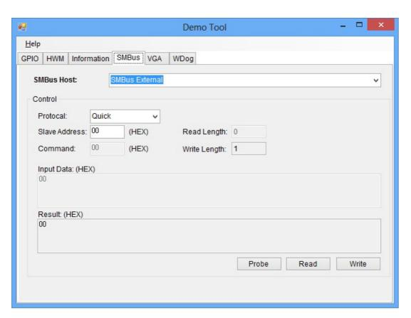
When the application has executed, you can click the radio button to choose to test each access mode, i.e. Access a byte, Access multiple bytes and Access a word. All data must be read or written in hexadecimal except the numbers for the radio button: Access multiple bytes mode must be written in decimal. You can test the functionalities of the watchdog as follows:
