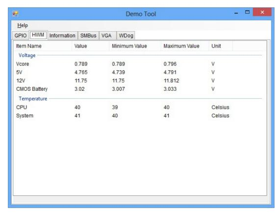
When the Monitor application is executed by clicking the button, hardware monitoring data values will be displayed. If certain data values are not supported by the platform, the correspondent data field will be grayed-out with a value of 0.
