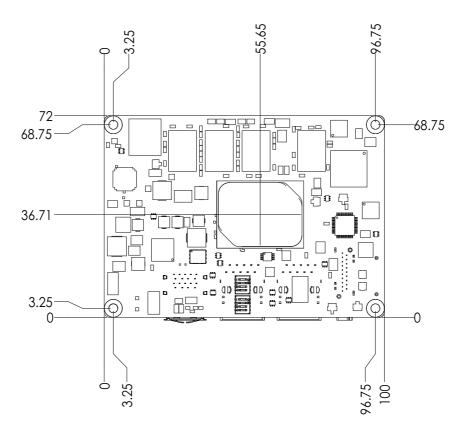
Figure 2.2 MIO-2361 Mechanical Drawing (Top Side)
