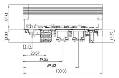
Figure 2.5 MIO-2361 Mechanical Drawing (Side View with Heatsink)
