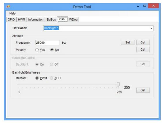
When the application is executed, it will display two blocks of VGA control functions. The application can turn on or turn off the screen shot freely, and it also can tune the brightness of the panels if your platform is supported. You can test the functionality of VGA control as follows:
