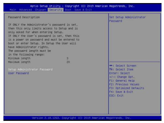
Select Security Setup from the MIO-2361 Setup main BIOS setup menu. All Security-Setup options, such as password protection and virus protection are described in this section. To access the sub menu for the following items, select the item and press <Enter>:
