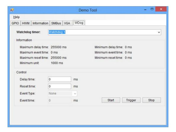
When the application is executed, it will display watchdog information in the WATCH-DOG INFORMATION group box. It displays max timeout, min timeout, and timeout steps in milliseconds. For example, a 1~255 seconds watchdog will have 255000 max timeout, 1000 min timeout, and 1000 timeout steps. You can test the functionality of the watchdog as follows:
