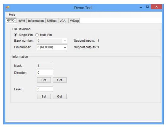
When the application is executed, it will display GPIO information in the GPIO INFORMATION group box. It displays the number of input pins and output pins. You can click the radio button to choose to test either the single pin function or multiple pin functions. The GPIO pin assignments of the supported platforms are located in Appendix B.
