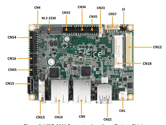
Figure 2.1 MIO-2361 Connector Locations (Bottom Side)
