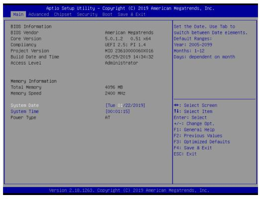
AMI BIOS ROM has a built-in Setup program that allows users to modify the basic system configuration. This information is stored in battery-backed CMOS so it retains the Setup information when the power is turned off.
